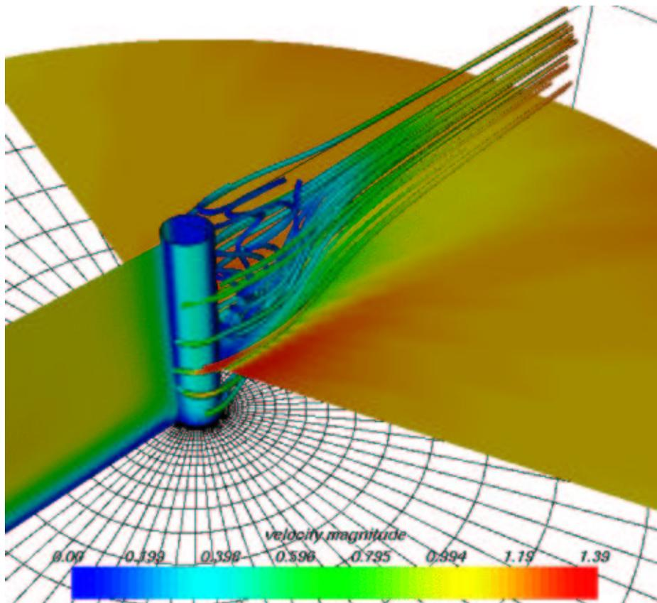
Figure 1: This figure shows stream-tubes for flow past a cylinder placed on a flat plate. Also shown are various cut planes that are colour mapped as per the velocity magnitude. One of them is a little away from the cylinder surface. The grid being used on the floor is also seen. The data used is courtesy NASA and is distributed along with VTK.
