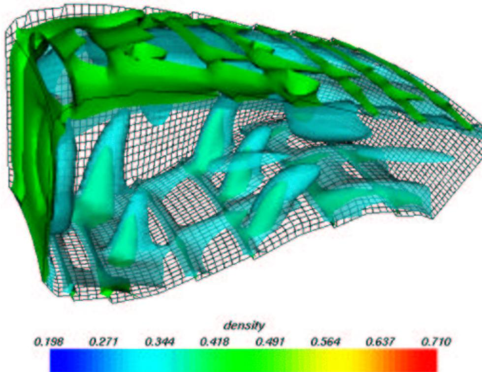
Figure 2: This shows a pair of iso-surfaces of density for flow inside a combustion chamber. Also shown are the structured grid planes that are used for the computation. This data is also courtesy NASA and is distributed along with VTK.
